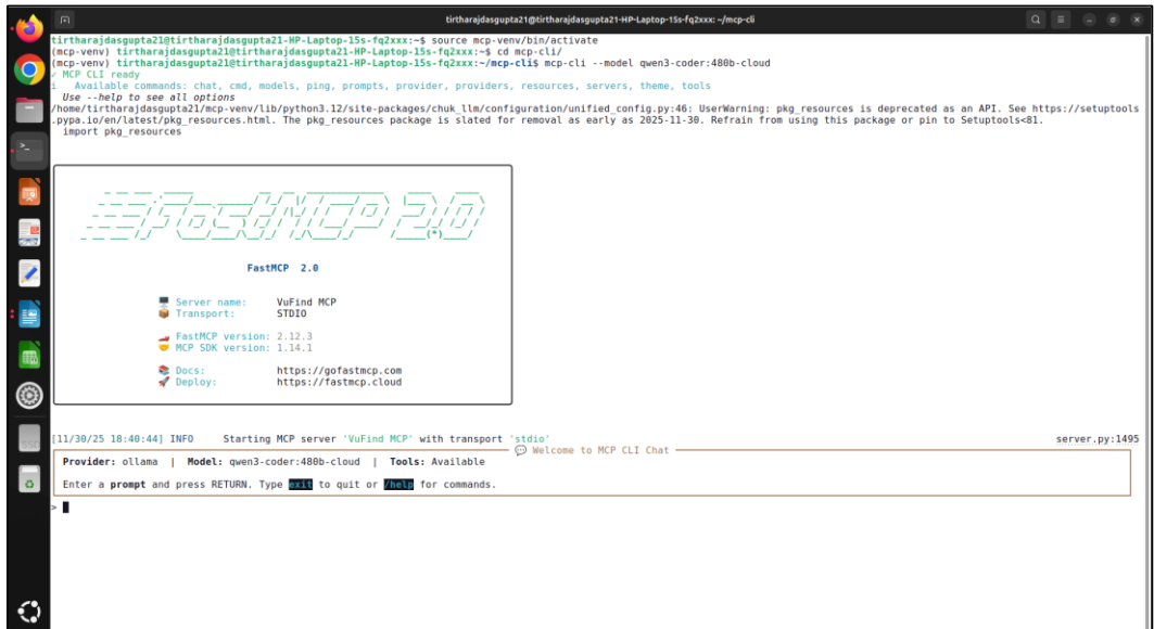
Figure 2 : Running the MCP CLI through the Linux Terminal while using Ollama, Qwen3 Coder cloud model and the MCP server for VuFind
